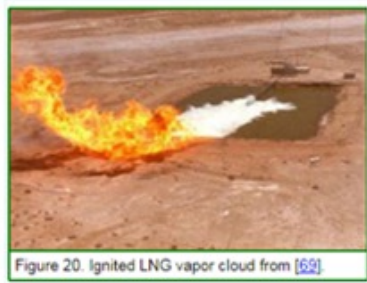
Figure 20. Ignited LNG vapor cloud from [62].
