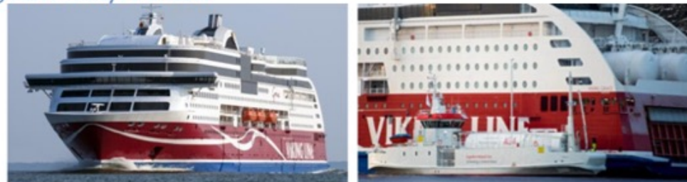
Fig.2.3 and 2.4 – MV Viking Grace. With a dedicated LNG bunker vessel (AGA Seagas 11 ), alongside in LNG bunkering operation.
