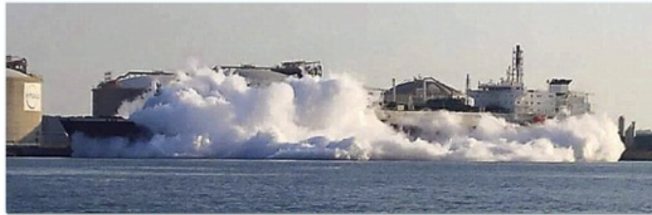
11 m3 of LNG released : No 1 tank overfilled and LNG was ejected via the forward vent mast raining down on the vessel's port side
