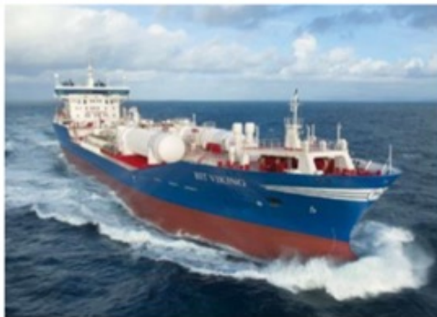
Fig 2.1 – MS BIT Viking – First ship converted to LNG power. [19]. The conversion involved installation of new dual fuel engines and LNG fuel system
