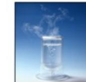
Figure 1. LNG "boiling" at atmospheric pressure and temperature (above -162°C) (CC-BY-SA via GFDL)
