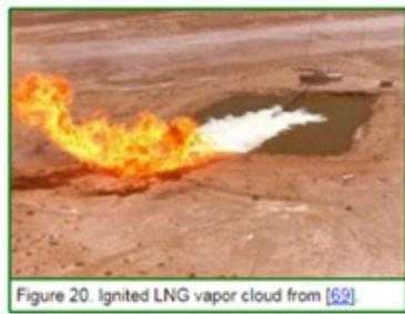
Figure 20. Ignited LNG vapor cloud from [62].
