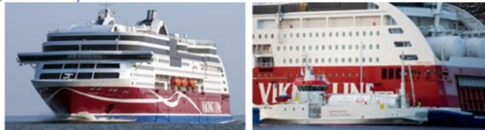
Fig.2.3 and 2.4 – MV Viking Grace. With a dedicated LNG bunker vessel (AGA Seagas<sup>11</sup>), alongside in LNG bunkering operation.
