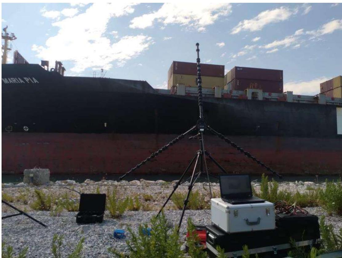
**Figura A. Misura 1.1, Acoustic camera.**
