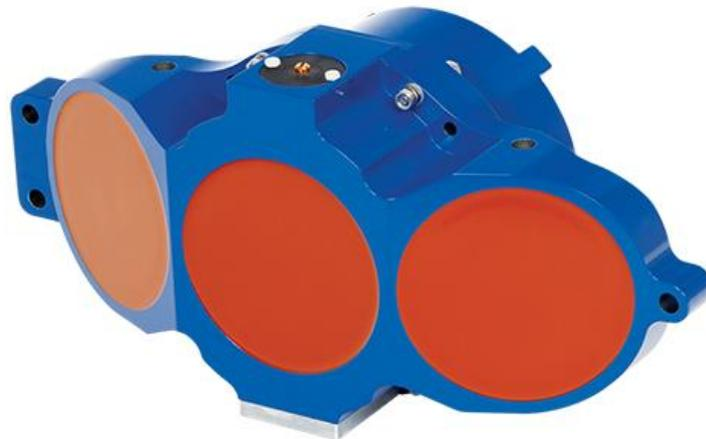
Fig. 2.3 Workhorse ADCP orizzontale (RD Instruments)
